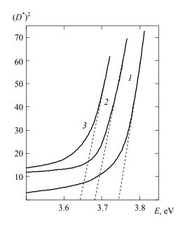
Fig. 1. Spectra of optical density of ZnS (1) and ZnS:Co samples 3 (2) and 4 (3).
