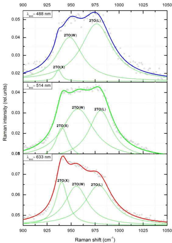
**Fig. 4 Normalized Raman two-phonon scattering for three different laser wavelengths for sample A. The calculated separate second-order modes are indicated by solid green line curve and the experimental data are plotted as colored bold line.**
