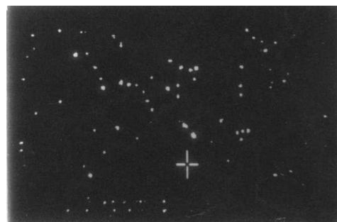
FIG. 1. Image of artificial stars given by the sensor (250x250 pixels)
